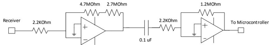
Figure 5. Custom built amplifier [1]
