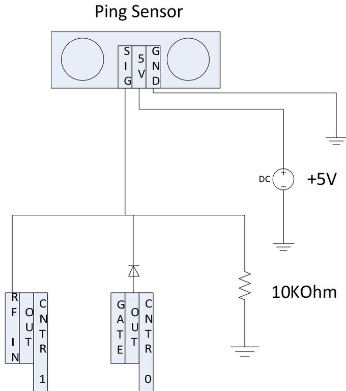
Figure 3. Ping sensor circuit [19]
