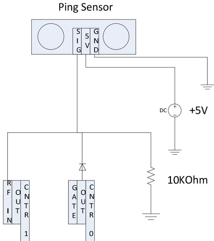
Figure 3. Ping sensor circuit [19]
